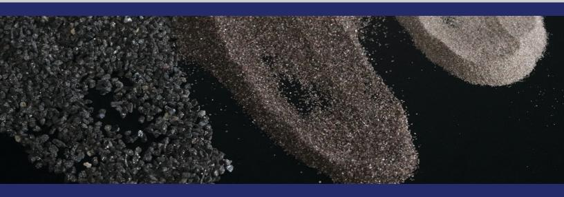
**RockRidge**<sup>®</sup> **Aluminum Oxide** is manufactured in an electric arc furnace that produces an extremely tough, long-lasting abrasive grain which is graded to macrogrit exacting standards. Aluminum Oxide can be repeatedly recirculated. It is also chemically stable.
